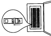
A WARNING HAZARD OF ELECTRICAL SHOCK! Before removing any access panels or servicing the water heater, make sure the electrical supply to the water heater is turned "OFF". Failure to do this could result in DEATH, SERI-OUS BODILY INJURY, OR PROPERTY DAMAGE.
